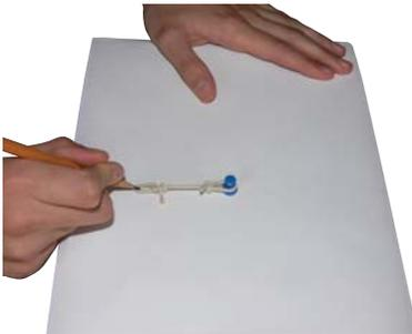
Put one loop over the push pin and put your pencil tip into the other loop.
