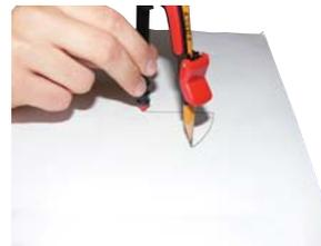
Hold the compass point at its end of the line segment as you rotate the compass to draw the circle.
